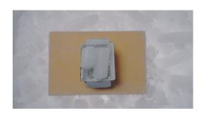
h. After **5 min**, remove mold B and check if the OCT is completely frozen and turns opaque, otherwise repeat f.
