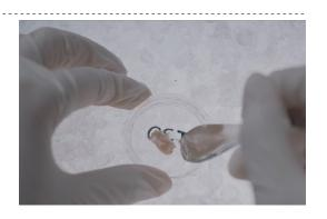
d. Remove any air bubbles using a syringe.
