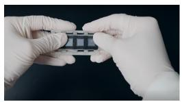
d. Press along both edges of the Stereoseq Slide Cassette to ensure the Stereoseq Chip Slide is locked in place.
