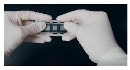
b. Lift the Stereo-seq Chip Slide from the side with the engraved label.
