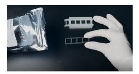
b. Pick up the Stereo-seq Slide Cassette and flip over. Insert the gasket into Stereo-seq Slide Cassette, ensuring the cutouts are aligned.
