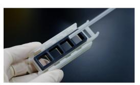
e. Pick up the Stereo-seq Chip Slide and flip over with the chip surface facing down. Align the engraved label with the long edge of the Stereo-seq Slide Cassette.
