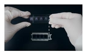
a. Make sure the chips are aligned within the empty space of the gasket and avoid touching the chip surface with the gasket or cassette during slide placement. Insert Stereo-seq Chip Slide under the bottom 4 tabs.
