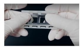
d. Use a power dust remover to blow off any debris on the gasket if necessary.
